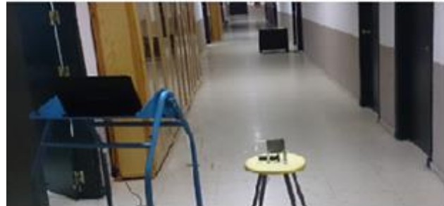
Figure 8 Test scenario. Assembly of the radar system with computer display of the data of speed and distance.
