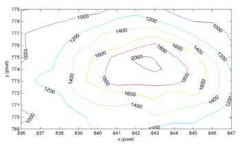
Figure 3 Level curves for the PSF of one of the images taken of the asteroid 2235 Vittore. Each curve indicates the intensity values registered in Analog Digital Units (ADU's). Given that the images were captured with a camera that has an analog to digital conversion of 16 bits in depth, the ADU's range is from 0 to 65535.
