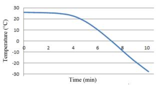
Figure 16 Freeze rate at 66 psi.
