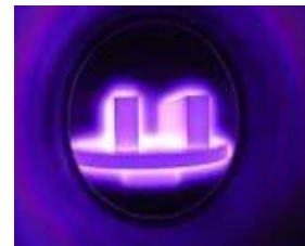
Figure 8. Observation of the nitriding process through the pyrex viewer. Prepared by the authors.
