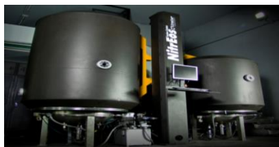
Figure 4. Plasma nitriding equipment NitrEos of Tratar S.A. Available at: http://www.tratar.com.co .
