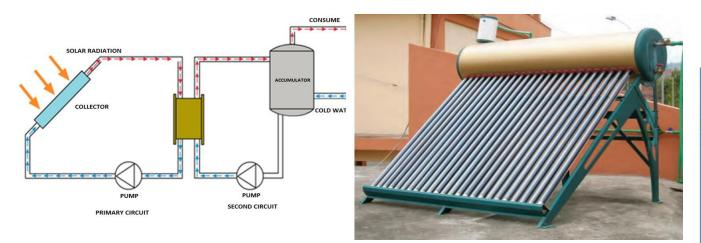
Figure 6. Scheme for solar water heater [13]
