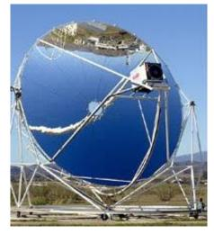
Figure 2. Parabolic dish type collector. [5]
