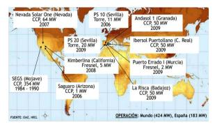
*Figure 12.* Thermo-solar projects in operation in the world. Taken from: [19] [20]
