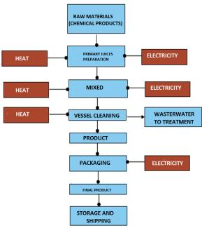
Figure 8. Manufacture of chemical products
