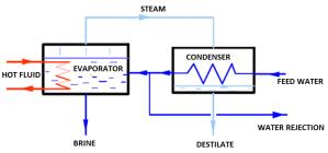
Figure 9. Operating scheme of water desalination
