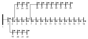
Fig. 5. 33-node radial distribution network. Source: Authors based on [30]
