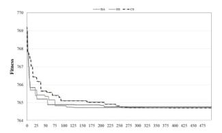
Fig. 6. Fitness reduction in the 33-node radial distribution network. Source: Authors
