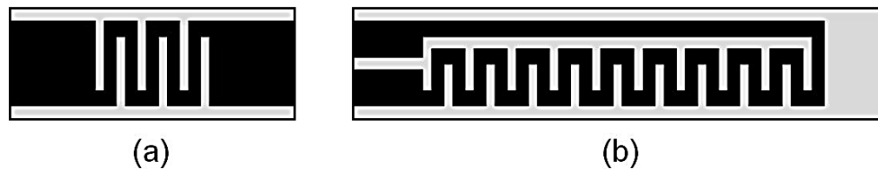
Fig. 5. Shape of heaters (dark areas) embedded in actuators: a) shorter, b) longer. Source: Authors.
