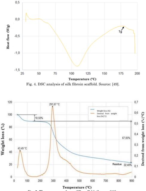
Fig. 5. Thermograms of pure SF scaffold. Source: [80].
