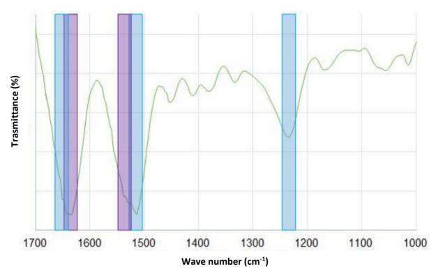
Fig. 2. FTIR spectra of electrospun silk nanofiber mat Source: [73].
