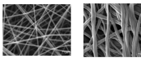
Fig. 1. Silk Fibroin (SF) nanofibers at concentrations of 13% wt. (a) Pure SF 146.58 ± 36.09nm,
