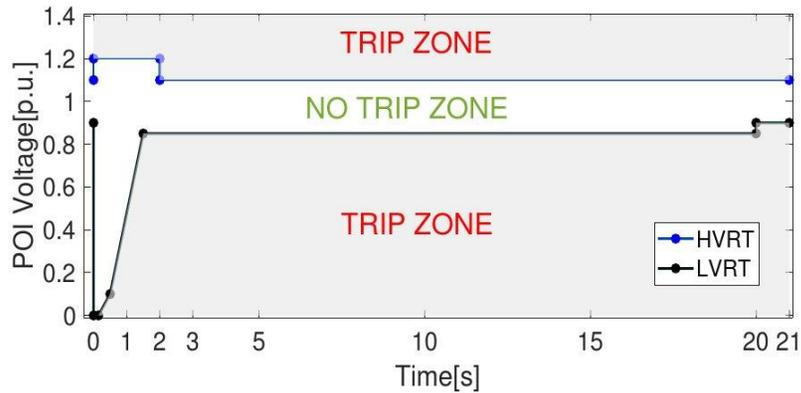
Figure 5. Fault ride through curve. Source: Created by the authors.
