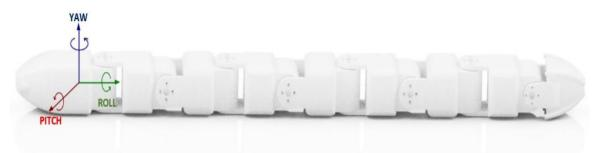
Figure 7. Prototype of the snake robot. Source: Created by the authors.
