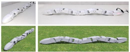
Figure 13. Rectilinear motion with the real robot and in simulation. Source: Created by the authors.
