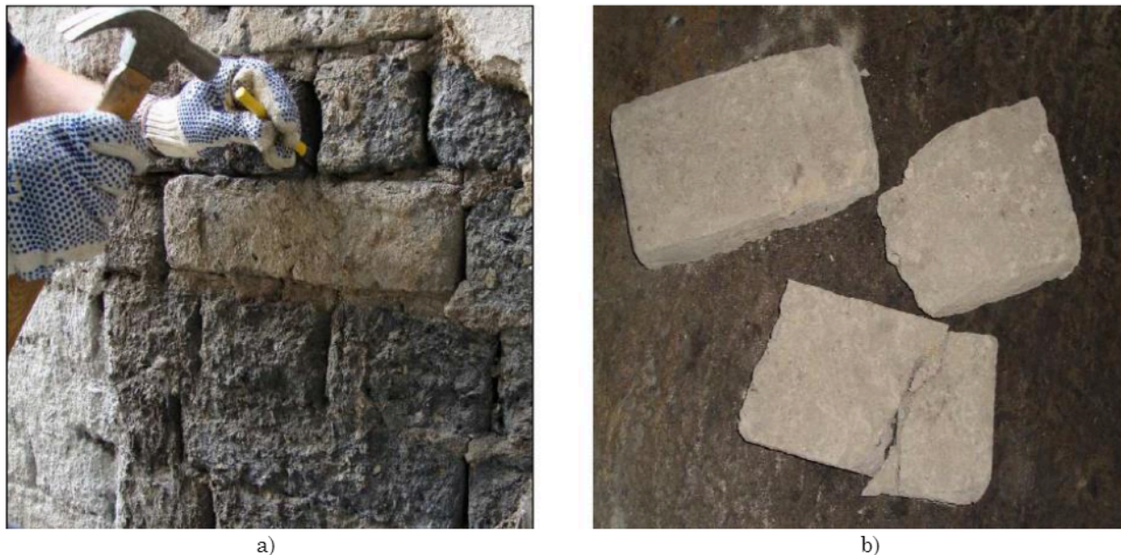
Figure 2. Samples of old adobe: a) recuperation of an adobe unit; b) recovered samples. Source: Created by the authors
