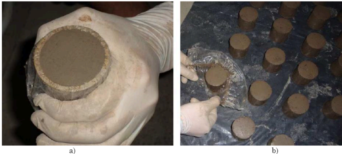
Figure 3. Samples of new adobe: a) preparation of the sample; b) air drying process. Source: Created by the authors
