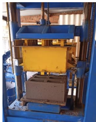
Figure 7. Blocks released from the vibro-compactor. Source: own work.
