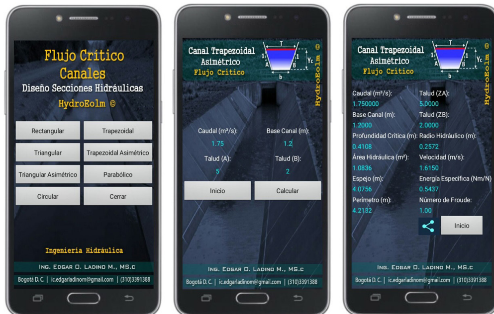
Figure 10. Asymmetric trapezoidal channel (Application critical depth solution)
